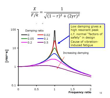
Differentiating w.r.t the frequency ratio r we obtain the value of r that makes the amplitude ratio has its maximum value.
